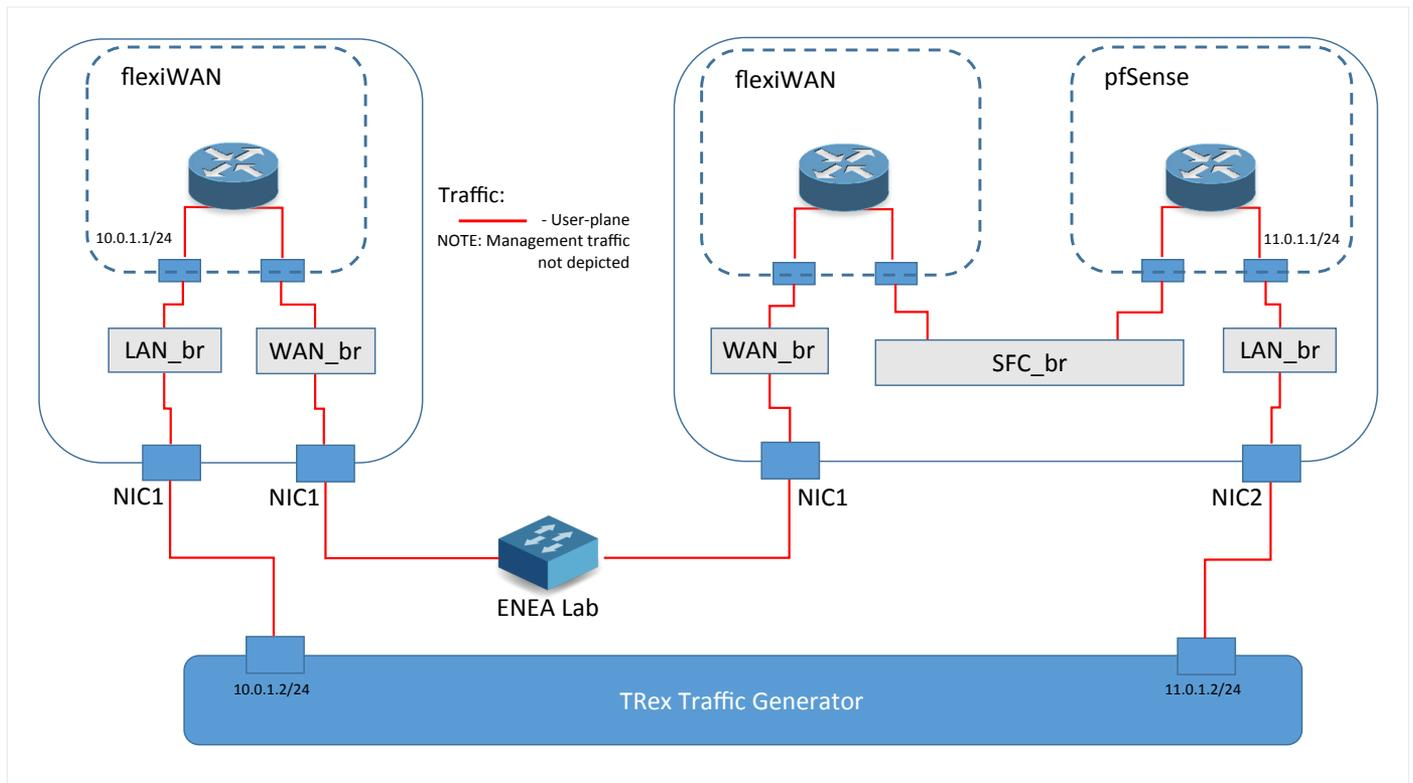
Figure 5. Service chain for test of SD-WAN and firewall services
