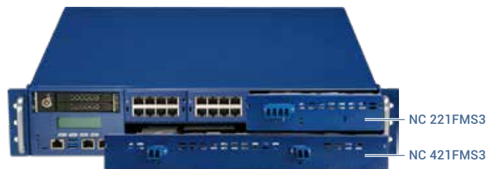
Figure 1. NVIDIA® Mellanox® ConnectX®-5-based 100G bypass LAN module in NSA 7146
