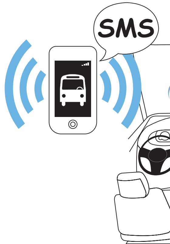
Figure 1: With integrated wireless network modem, the VTC 1000 in-vehicle computer can be activated by remote wake-up feature using SMS.
