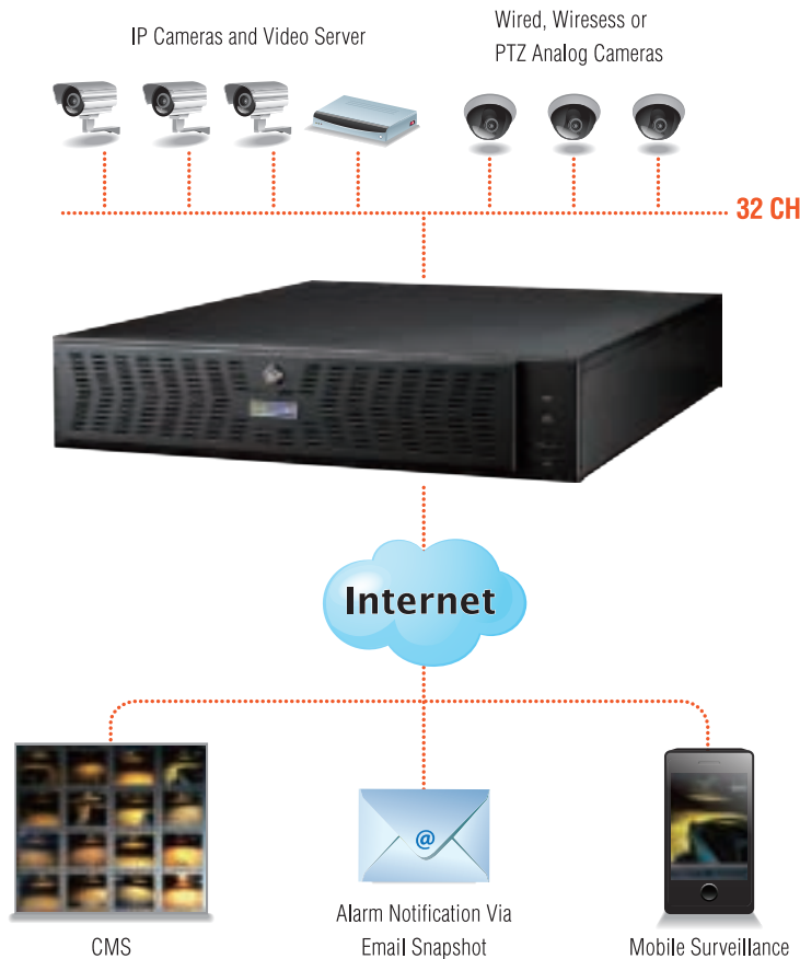
Figure 1. A hybrid NVR enables flexible management, intelligent alerts, and remote viewing for both analog and digital camera streams.
