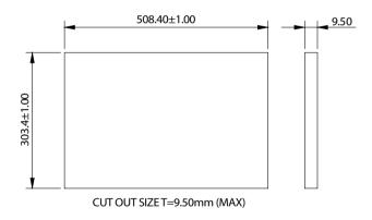
3. Slide the panel PC through the hole until it is properly fitted against the panel.
