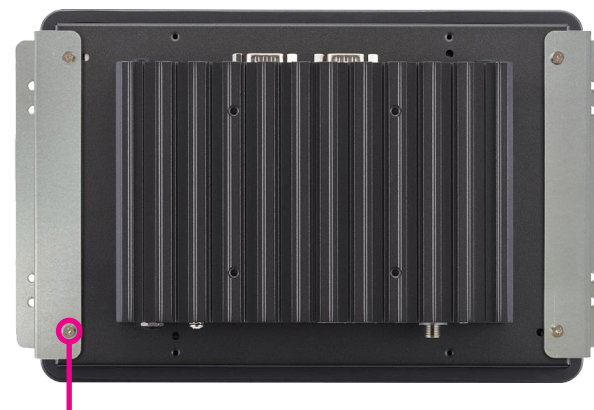
4 * Screws (F3x5 Nylok NI+Heat)
