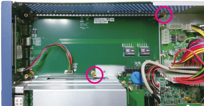
3. Align the mounting holes on the base plate to the copper standoffs.
