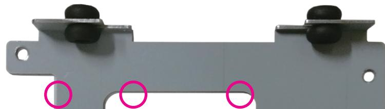
8. Repeat step 7 for securing the screws on the other side of the HDD tray.
