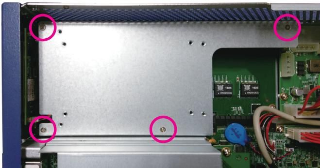
5. Align the mounting holes on the drive bay enclosure to the mounting holes on the drive bay bracket.
