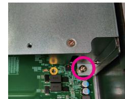
2. Remove the middle cover to access the CPU sockets.
