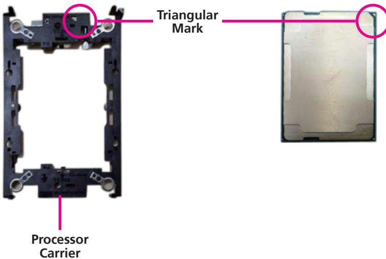
3. With the CPU placed into the processor carrier, install the CPU onto the CPU socket.
