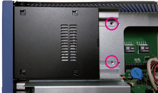
7. Repeat step 6 for securing the screws on the other side of the bracket.
