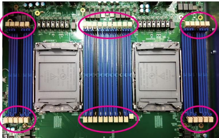
2. Insert the module into the socket at an 90 degree angle. Apply firm even pressure to each end of the module until it slips into the socket. While pushing the module into position, the locks will close automatically.
