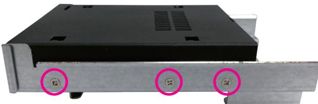
8. Fix the drive bay bracket to the base plate with screws.
