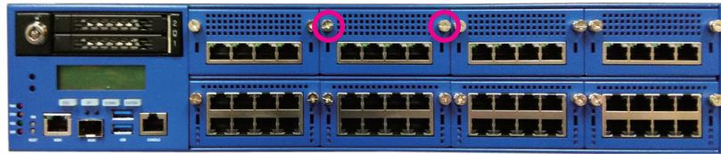
2. Use the handle provided, and insert the handle into the two holes on the LAN module.
