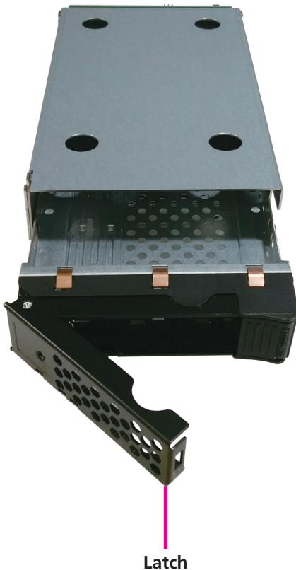
7. Place the SATA drive onto the tray and align the mounting holes on the drive with the mounting holes on the tray, then secure the drive in place with screws.
