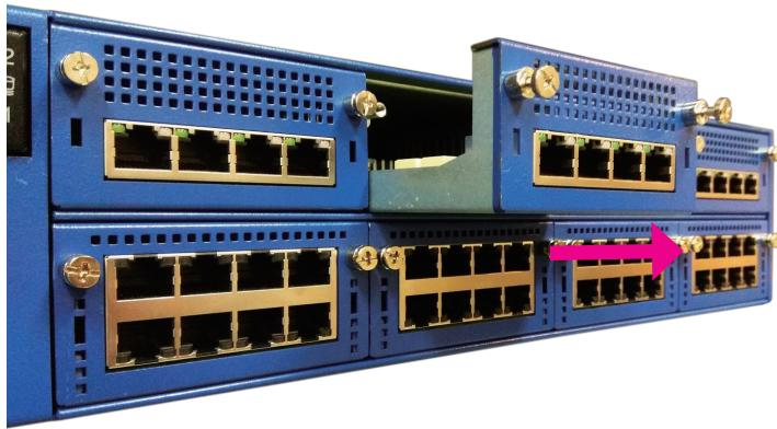
4. Insert the new LAN module into the slot and secure the module with the two screws.
