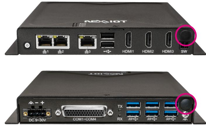
2. Insert the SMA antenna jack end of the cable through the antenna hole, and insert the 2 rings (ring 1 and ring 2) and two washers back to the antenna jack.
