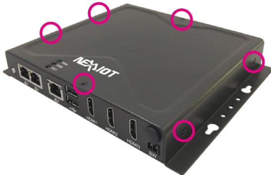
2. With the screws removed, lift up the cover and remove it from the chassis.
