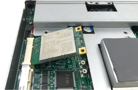
3. Push the module down and secure it with a screw.
