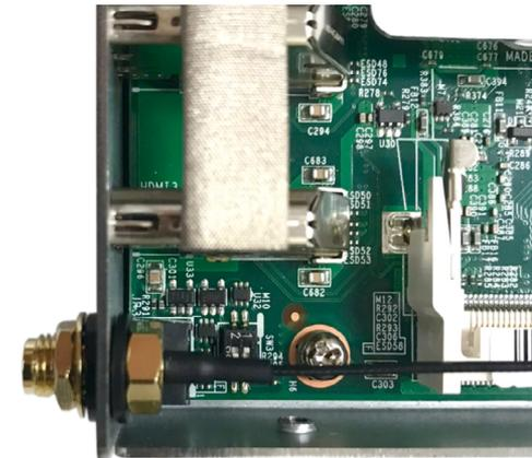
4. Connect the external antenna to the antenna jack.
