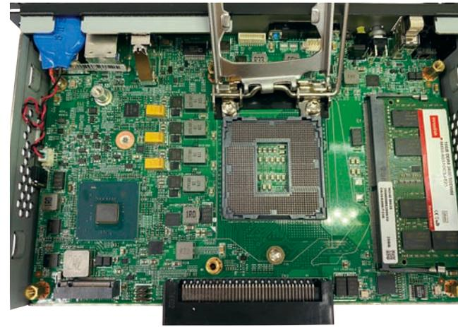
3. Insert the CPU into the socket. The triangular edge on the CPU must align with the corner of the CPU socket shown on the photo.
