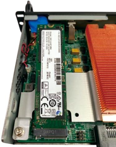
4. Push the module down and secure it with the screw removed in step 2.
