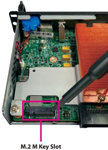
2. Remove the screw on the copper standoff. Put the screw in a safe place for later use.
