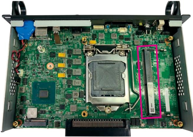
4. Insert the module into the socket at a 30-degree angle. Then push the module down until the clips on both sides of the socket lock into position. You will hear a distinctive “click” sound, indicating the module is correctly locked into position.
