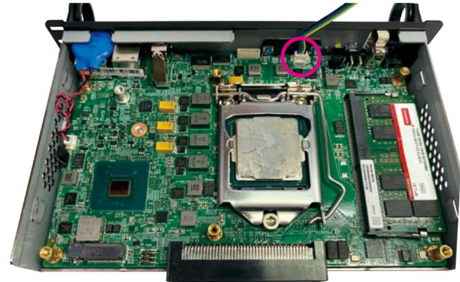
3. Locate the SO-DIMM socket.
