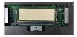
5. Refer to step 1 to secure the SO-DIMM cover back in place using the screw.
