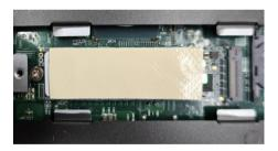
6. Refer to step 1 to secure the M.2 cover back in place using the screw.
