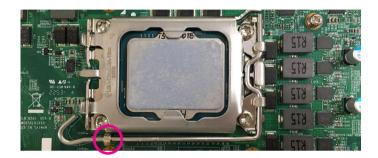
6. Applying thermal paste before assembling the heatsink to ensure proper heat transfer between the CPU and the heatsink.
