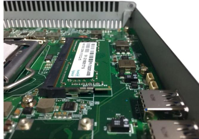
3. Open the bottom cover for installing the 2nd SO-DIMM memory module.
