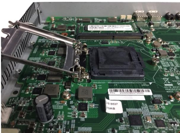
2. Insert the CPU into the socket. The triangular edge on the CPU must align with the corner of the CPU socket shown on the photo.
