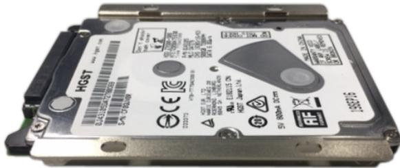
3. Place the SATA drive in the chassis and connect the SATA data connector, then use screws to secure the drive in the chassis.
