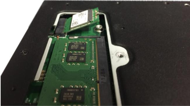
4. Secure the module with mounting screws and attach one end of the RF cables onto the module.
