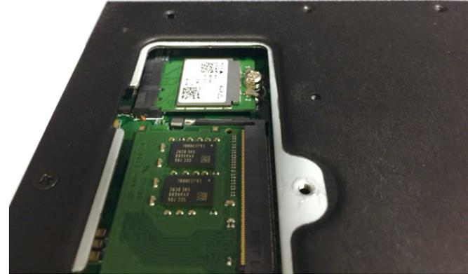
5. Insert the antenna jack end of the cable through the antenna hole.
