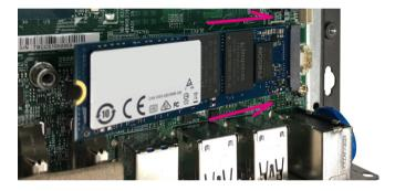
3. Push the M.2 module down and secure it with the screw that was removed from step 1.
