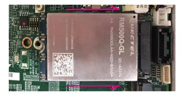
3. Push the M.2 module down and secure it with the screw that was removed from step 1.
