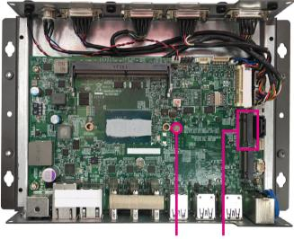
Screw for M.2 Key B M.2 Key B slot
