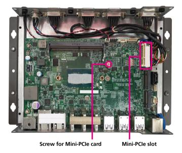
2. Insert the WiFi module into the mini PCIe slot at a 45-degree angle until the gold-plated connector on the edge of the module completely disappears into the slot.
