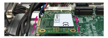
3. Push the WiFi module down and secure it with the screw that was removed from step 1.
