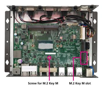
2. Insert the M.2 module into the M.2 Key M slot at a 45-degree angle until the gold-plated connector on the edge of the module completely disappears into the slot.
