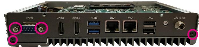
3. Secure the bottom cover to the chassis with four screws, then secure the wall mount bracket.
