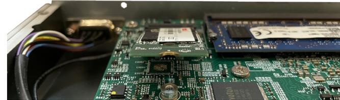
3. Push the module down and secure it with the screw that was removed from step 1.
