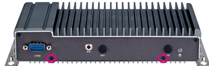
3. With the screws removed, lift up the cover and remove it from the chassis.
