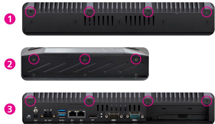
2. With the screws removed, lift up the cover and remove it from the chassis.
