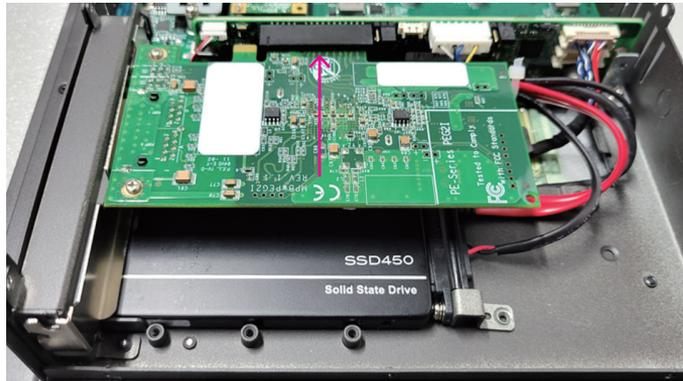
4. Lock the bracket of the PCIe card into the chassis.
