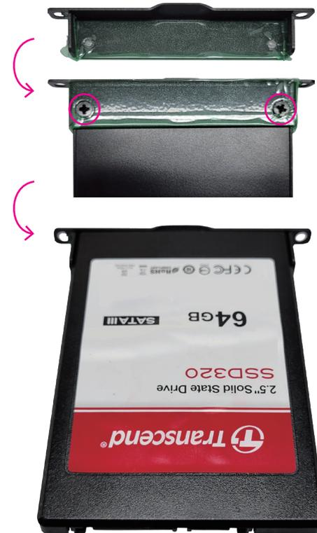
4. Insert the SSD with the tray installed into the system.
