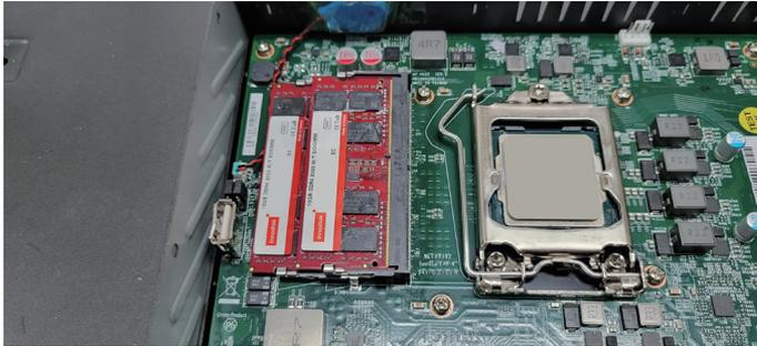
4. Attach the thermal pad (refer to the red square below) provided in the accessory box for the memory module on the top cover, ensuring it is evenly and securely attached, and remove the protective film before use. The blue square marks the area where the thermal pad for the mini-PCle/M.2 module should be attached.
