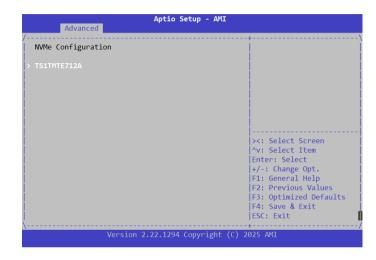
The NVMe device appears when plugged in. Press Enter for more configurations.
