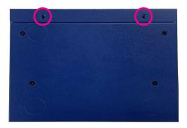
2. Push the cover outwards and lift up the cover to remove it.
