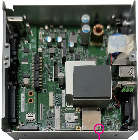
Secure the wireless LAN Module
