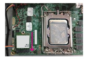
3. Push the Wi-Fi module down and fasten an M.2 mounting screw into the mounting hole to secure the module.
