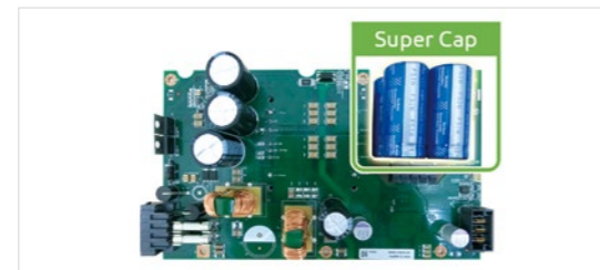
Protection for voltage dips
