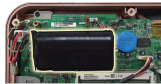
Back-up battery provides uninterrupted power
