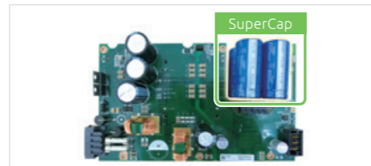
Protection for voltage dips
