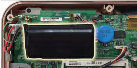
Back-up battery provides uninterrupted power
