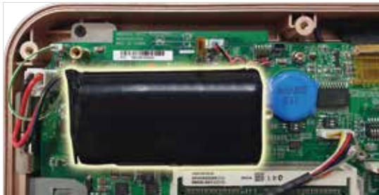
Back-up battery provides uninterrupted power
