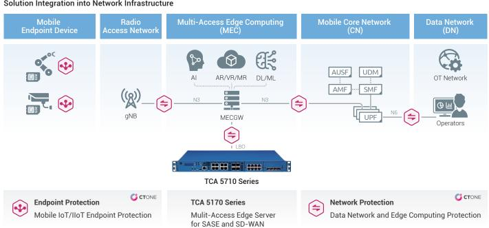
CTOne's virtualized private 5G security was installed on NEXCOM's TCA 5170, and units were further integrated at strategic points within the existing network architecture to provide real-time threat detection, intrusion prevention, and data encryption capabilities.
