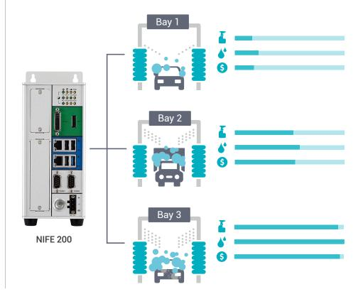
NEXCOM's PC-based controller with CODESYS Control RTE as the Modbus TCP and Modbus RTU controller can be in charge of a myriad of interfaces through all stages of three different washing lines while utilizing water resources more appropriately.
