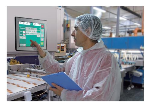
NEXCOM's EtherCAT-enabled solution with CODESYS software unifies the previous communication from Modbus RTU and CT Net by performing as controller and HMI at the same time, reaching higher data transfer speed to smooth the packing course.
