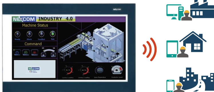
Figure 4. The NIFE 300's JMobile Suite is an HMI solution enabling local control and remote monitoring.
