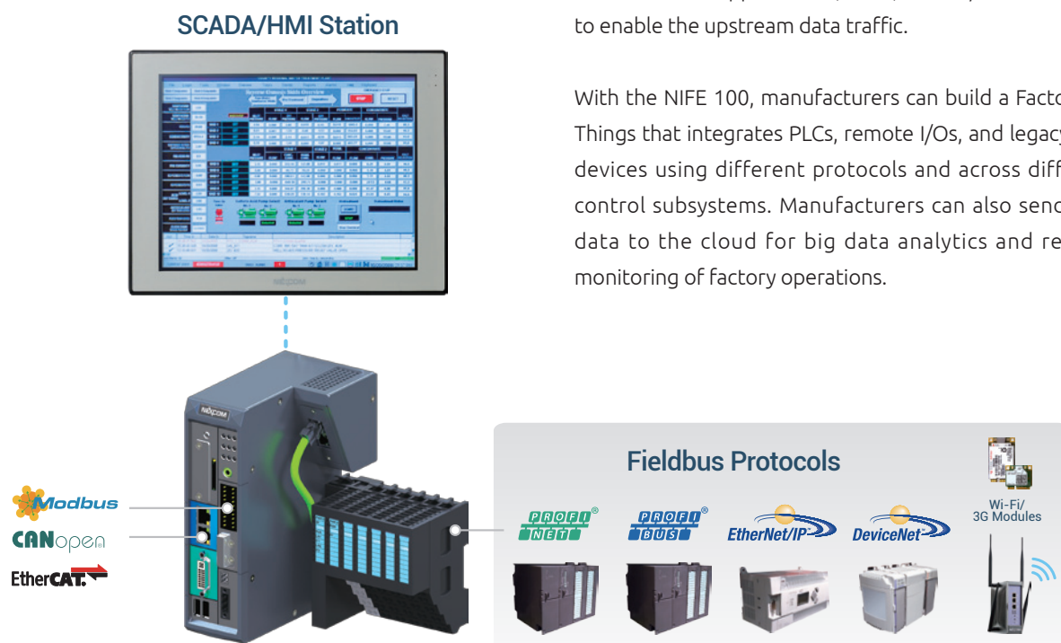
Figure 2. To aggregate field data, the NIFE 100 supports fieldbus communication and 3G/LTE/Wi-Fi networking at the same time.
