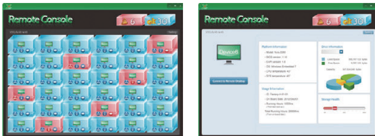
Figure 3: NEXCOM XCare gives alerts on issues across the factory (left). Operators can zoom in on individual systems (right) to quickly investigate and repair problems.
