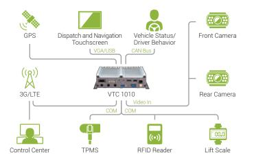
which residence it belonged to. The information can now be digitally processed by the VTC 1010 connected to lift scales, GPS, RFID readers and cameras, allowing operators to easily and accurately calculate bills for each residence, and provide proof of collection images taken by cameras.
