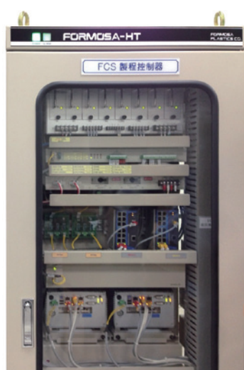
Figure 2. The FORMOSA-FX* system uses NEXCOM NISE* 3660 as a DCS controller.
